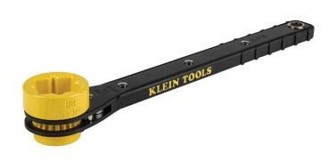
The Slim Ratcheting Lineman Wrench works on four different square sizes, covering all of the common utility pole hardware. The long handle provides plenty of leverage and a tight ratcheting mechanism increases efficiency. The high visibility yellow socket includes a bolt-through design, enabling use on long bolts. Handle is fully integrated for durability.
