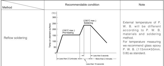
\*When performing reflow soldering, an appropriate coating thickness of cream solder is 0.10 to 0.15 mm.
