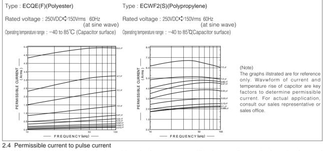
•When used in switching circuits or snubber circuits a momentary high current pulse may curse local heat generation which may despite the evaporated. Film causing the capacitance value to deteriorate or an open circuit condition.
