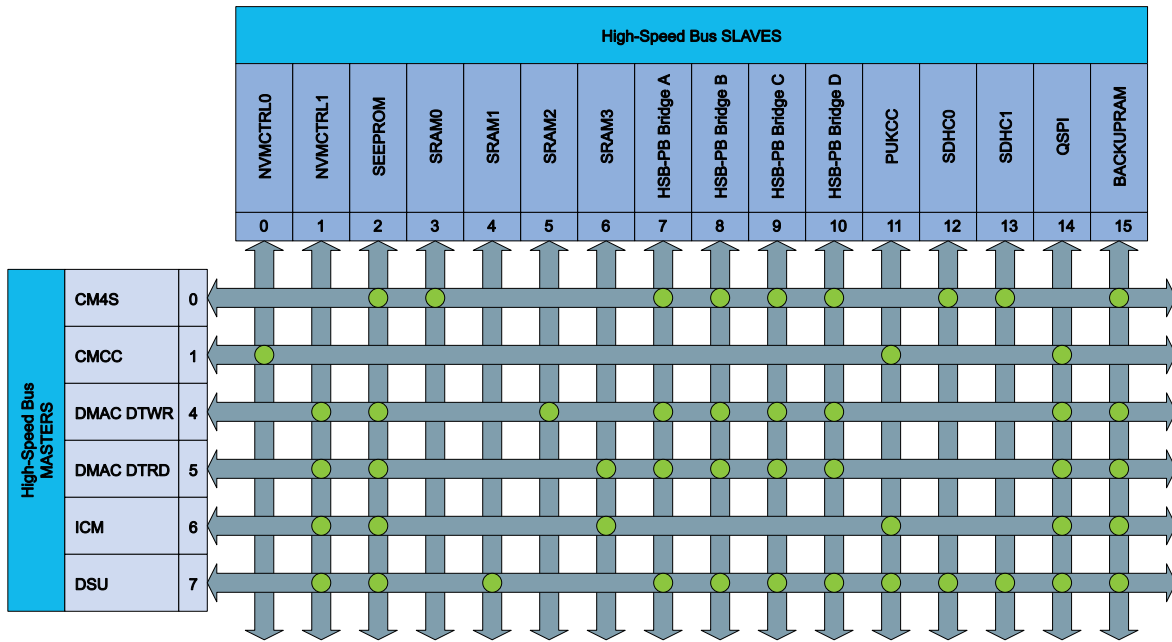
Figure 10-1. Master-Slave Relations High-Speed Bus Matrix
