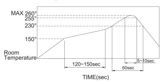
The condition mentioned above is the temperature on the Cu foil of the PCB surface. There are cases where board's temperature greatly differs from switch's surface be used not to allow switch's surface temperature to exceed 260°C.
