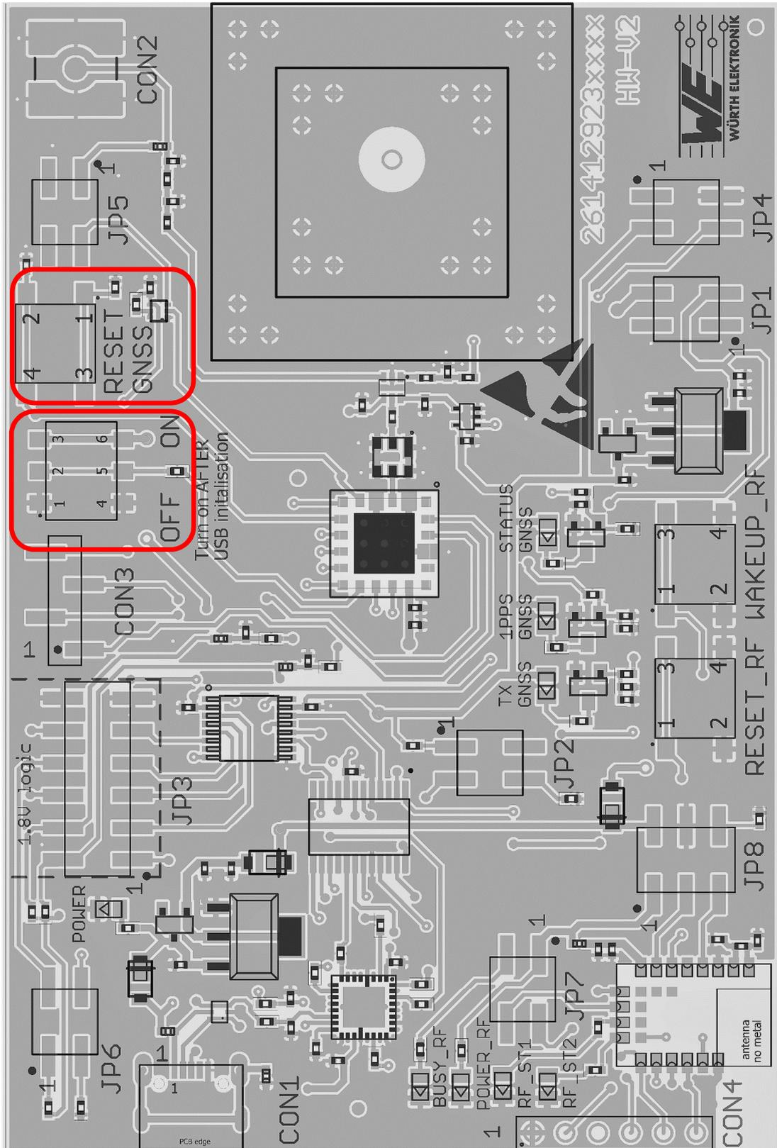
Figure 6: Switches and Buttons
