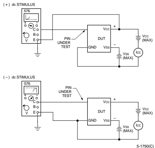
Figure 4. Test 1: Equipment Hookup: I/O Stress
