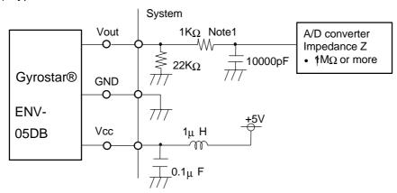
Note1) The value of this resistance should be 1/1000 or less of impedance of A/D converter
