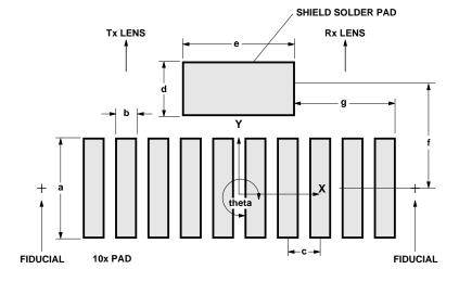
$\label{eq:Figure 2.} \textbf{Figure 2. Top view of land pattern.}$
