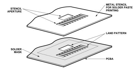
Figure 1. Stencil and PCBA.
