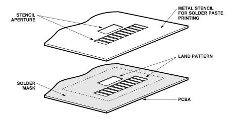
Figure 1. Stencil and PCBA.
