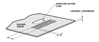
Figure 4. Solder paste stencil aperture.
