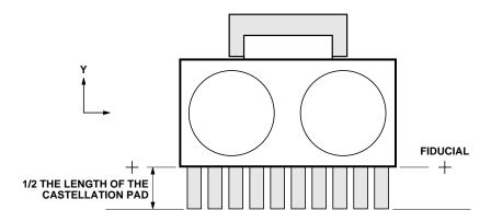
Figure 2. Section of a castellation in Y-axis.
