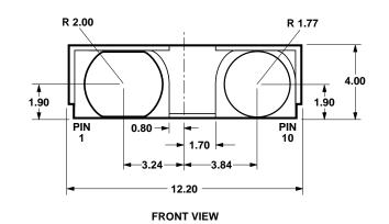
ALL DIMENSIONS IN MILLIMETERS (mm).
