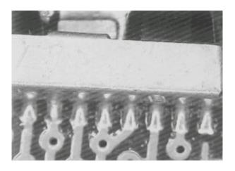
Picture 4. Unit self-aligns after reflow.
