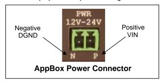
Listed below are the steps to attach the AppBox Power Supply to an AppBox:
