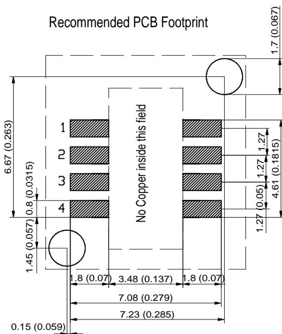
Figure 4 Footprint dimensions are in mm (inch)
