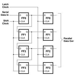
Shift-Register Output with Shiftout. The most basic use for Shiftout is to Figure 3. A shift register plus a latch makes a serial-to-parallel converter.
