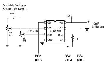
Figure 6. Schematic for LTC1298.BS2.
