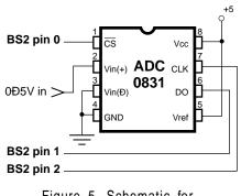
Figure 5. Schematic for ADC0831.Bs2.
