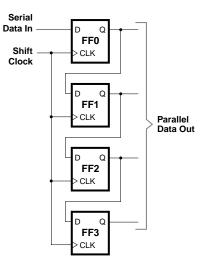
Figure 2. Serial shift register.
