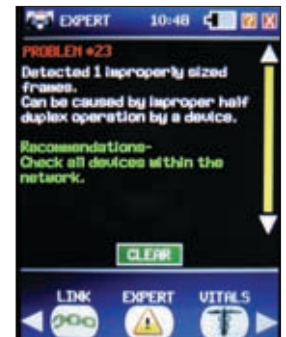
The Expert feature provides solutions to common network problems.
