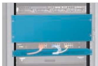
Filler Panels and Air Dams keep cool air in the front of the cabinet where it is needed by equipment, and keep warm air from escaping to the front of the cabinet.
