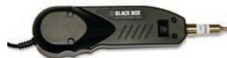
End-face inspection, using either a handheld optical or video microscope (the latter is shown here), should be done both during and after termination to check for contaminated or improperly polished connector end-faces.
