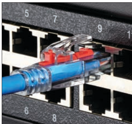
A locked-down cable with Pin inserted in the boot. To unlock, insert the Key into the Pin until it clicks. Pull the Pin back and lift the Key to release.
