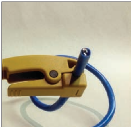
Cable being stripped.
