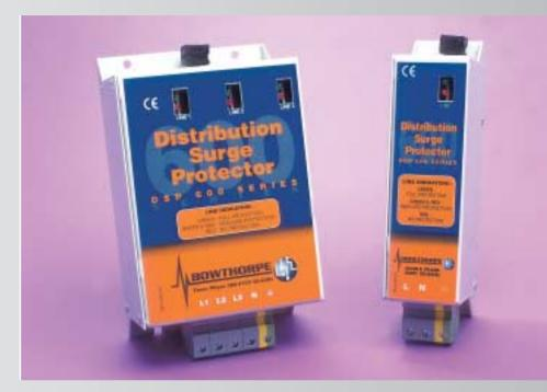
open or close when the first stage protection is lost, (Red and Green LEDs on), and these can be used to activate a remote indicator such as a lamp or an audible alarm. The switching contacts are completely isolated from the supply and may be used for AC mains voltage 230V RMS 200mA or 30V DC 2 Amp loads.
