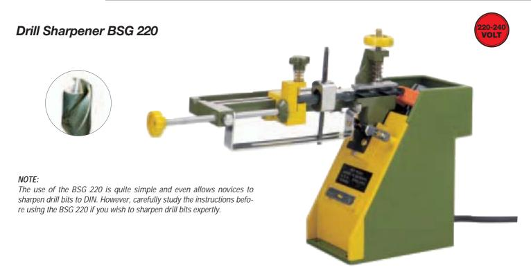
The operation is relatively simple, enabling everybody to sharpen standard 118° HSS, CrV and tungsten bits of 3 - 13mm diameter professionally.
