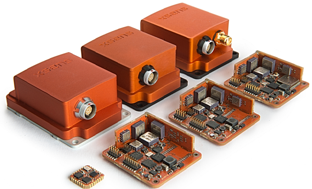
Figure 1: Xsens Motion Tracker products for industrial applications (MTi). In the bottom row, from left to right - the 1-series module, OEM version of 10-series, 100-series and MTi-G-710. In the top row, from left to right - the encased version of 10-series, 100-series and MTi-G-710.
