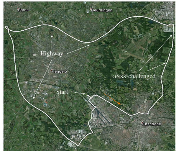
Figure 8: AUTOMOTIVE TEST: The automotive test trajectory run done near Enschede, The Netherlands. The MTi-G-7XX trajectory shown is as output by the KMZ exporter of the MT manager. The start and end points of the test run are the same as indicated in the figure. The GNSS-challenged segments point to areas with thick tree canopy.
