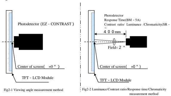
Fig2 Optical characteristics measurement method
