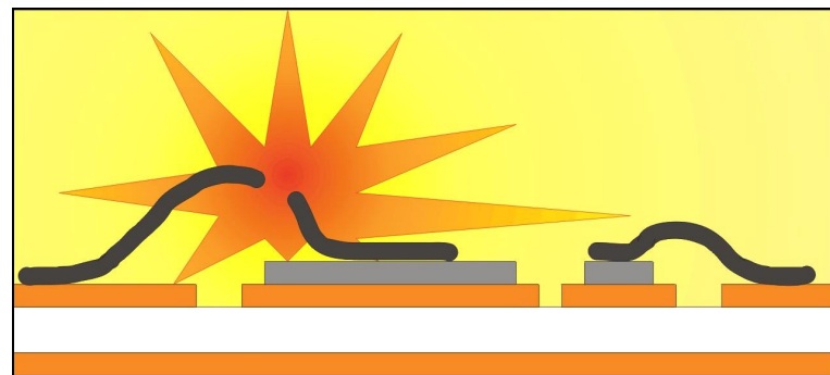
Fig. 5-4 Sketch of high energy plasma caused by bond wire melting
