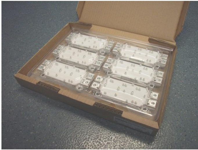
Fig. 12-1 Cardboard box with SEMiX in transparent ESD tray; dimensions: 350 x 280 x 50 mm 3 (l x w x h)
