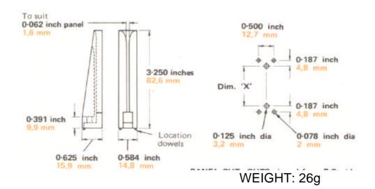
PANEL CUT-OUTS viewed from P.C. side Dimension 'x' to be fixing centres of any P.C. connector Location dowel holes to be within 0.05mm dia of true position
