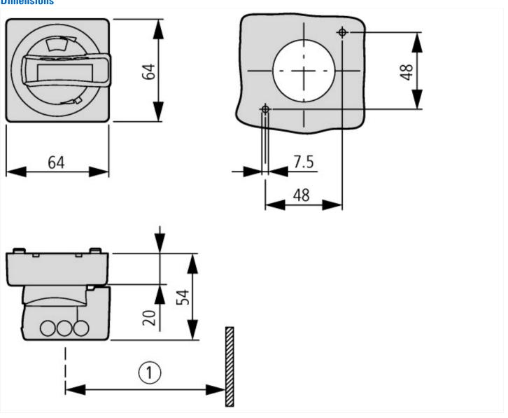
Mounting depth: 125 to 240 mm from the top edge of the top-hat rail to the front edge of the cabinet door/cover
