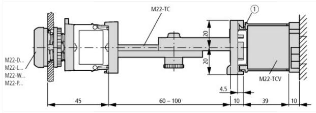
Pushbuttons and indicator lights with M22-TC telescopic clip and M22-TCV extension 1 Top-hat rail to IEC/EN 60715
