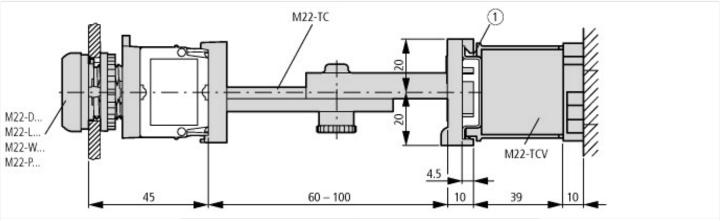
Pushbuttons and indicator lights with M22-TC telescopic clip and M22-TCV extension 1 Top-hat rail to IEC/EN 60715
