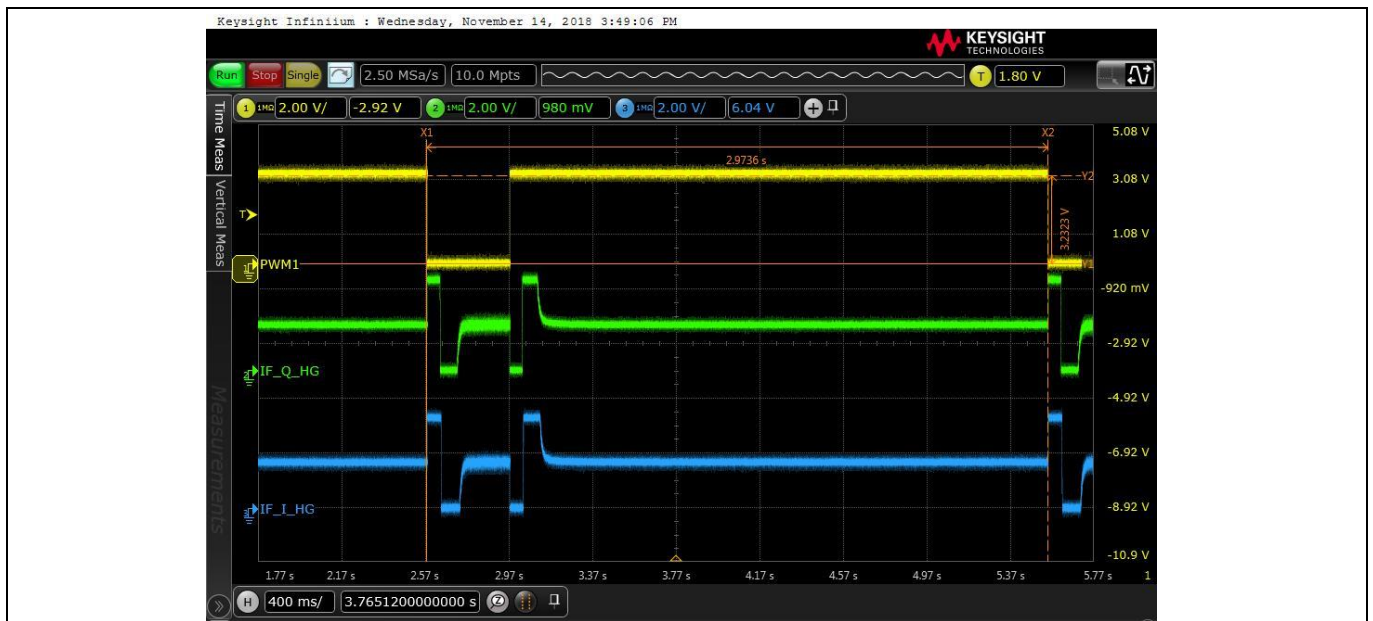
Figure 18 PWM1, IF_Q and IF_I signals for on-time = 400 ms and frame interval time = 3000 ms
