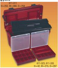
Tough polypropylene tool box with snap action catches and padlock facility, also optional webbing shoulder strap. Special locking handle prevents lid from opening when in upright position. Lift out tray will accept up to two 9 or 15 division compartment boxes supplied separately.
