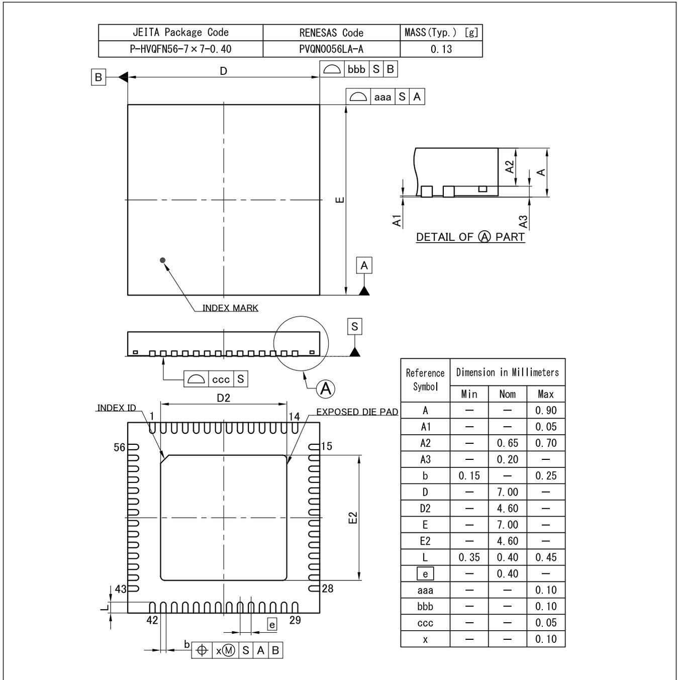
Figure 2.5 QFN 56-pin
