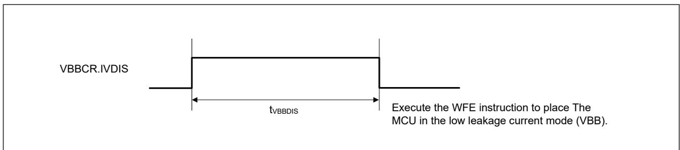
Figure 2.52 Internal voltage discharge time
