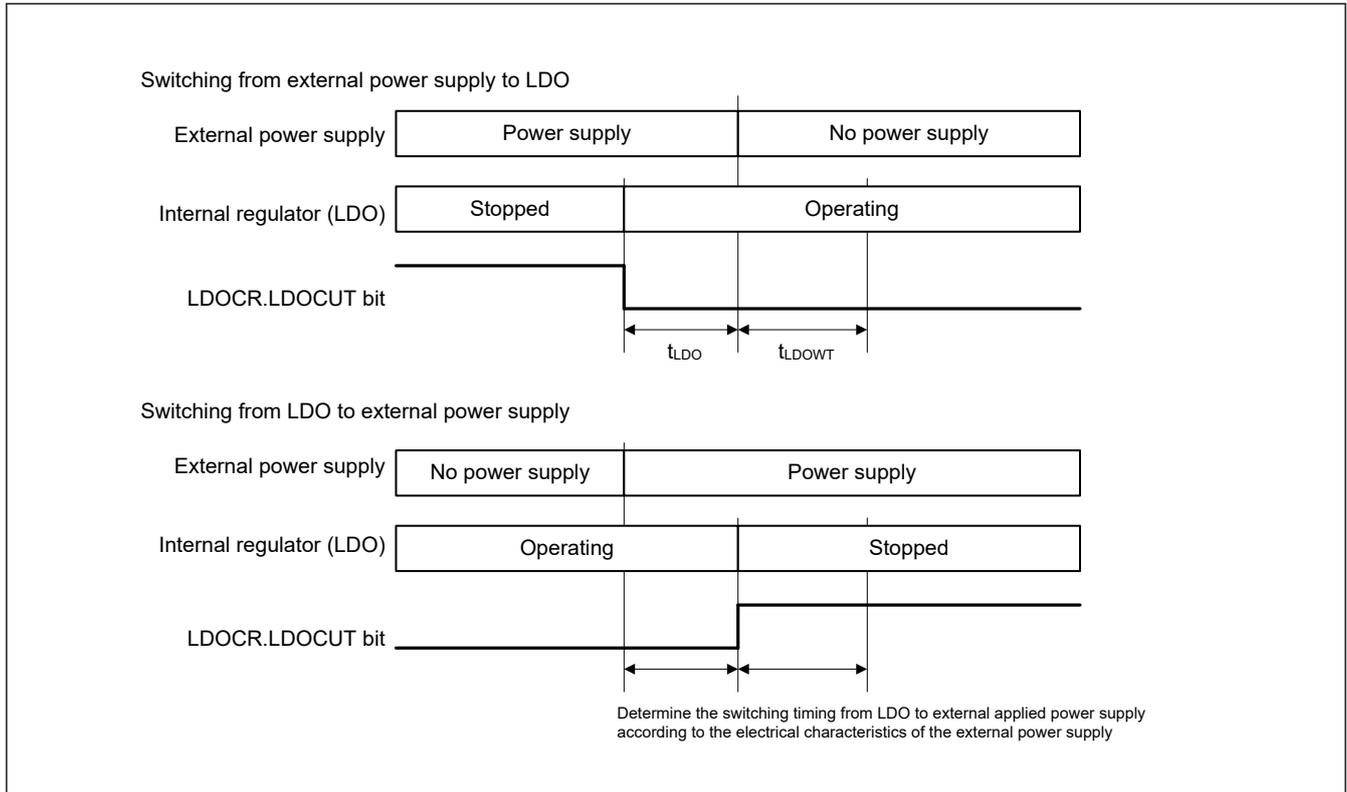
**Figure 2.2 Switching timing between external power supply and LDO**
