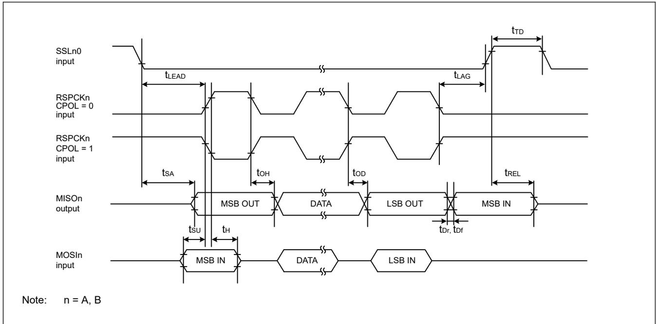
Figure 2.34 SPI timing (slave, CPHA = 0)
