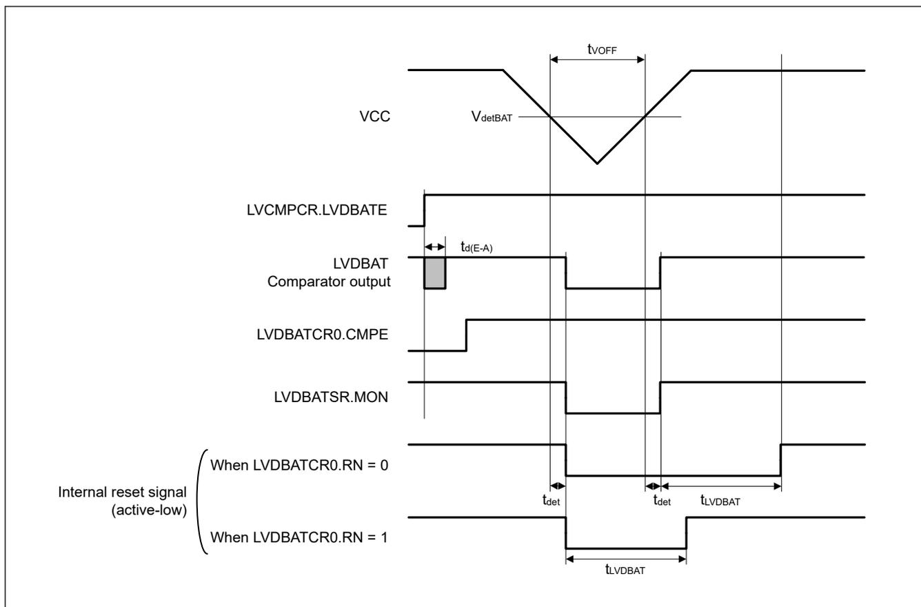
Figure 2.47 Voltage monitoring BAT circuit detection voltage timing (V<sub>detBAT</sub>)
