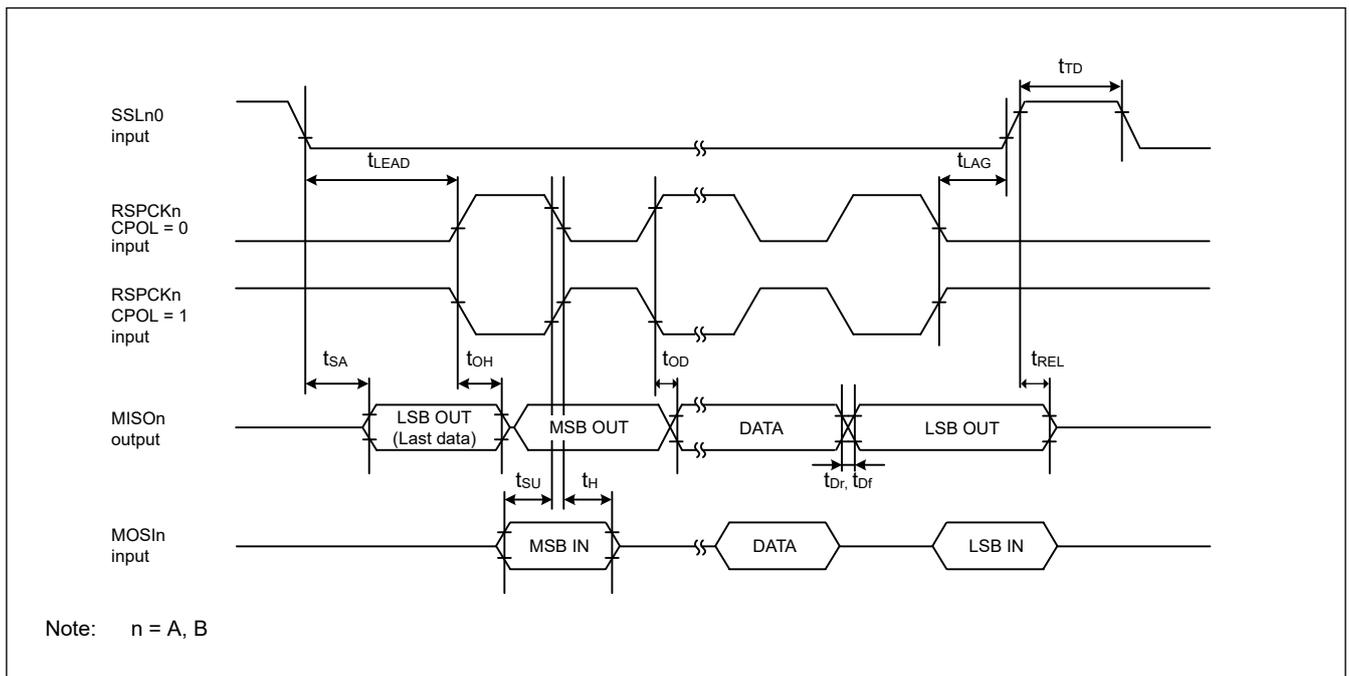
Figure 2.35 SPI timing (slave, CPHA = 1)
