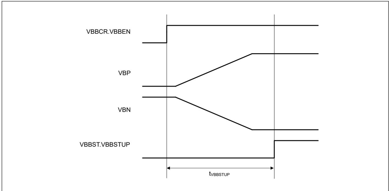
Figure 2.51 VBBC initial setup timing
