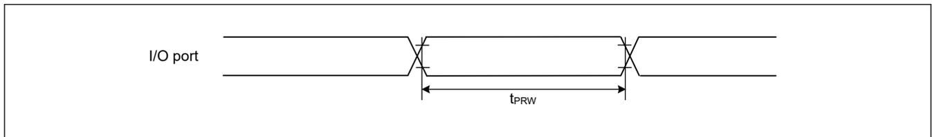
**Figure 2.16 I/O port input data pulse width**
