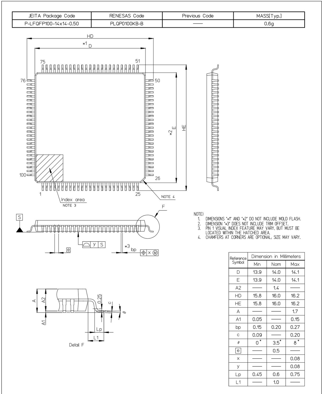
Figure 2.1 LFQFP 100-pin
