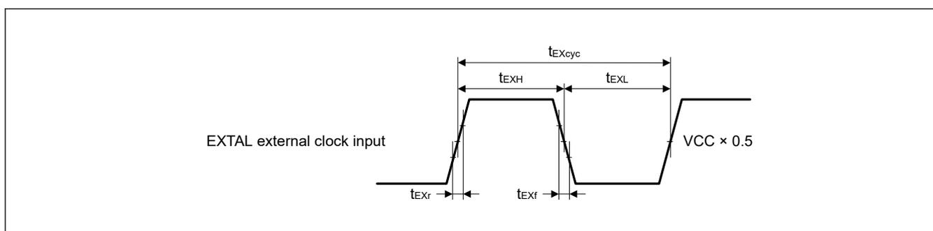
**Figure 2.3 EXTERNAL external clock input timing**
