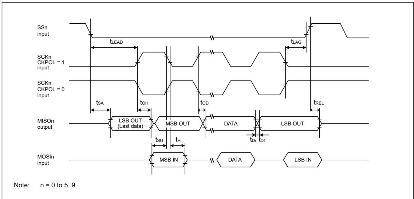
Figure 2.27 SCK input/output timing (simple SPI mode) (slave, SPMR.CKPH = 0)
