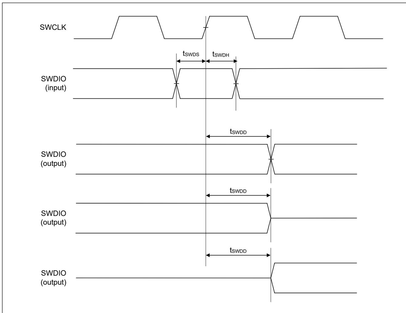
Figure 2.57 SWD input/output timing
