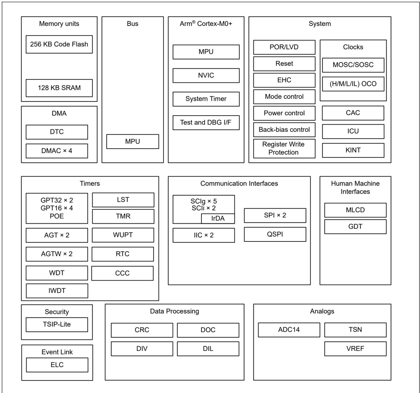
Figure 1.1 Block diagram
