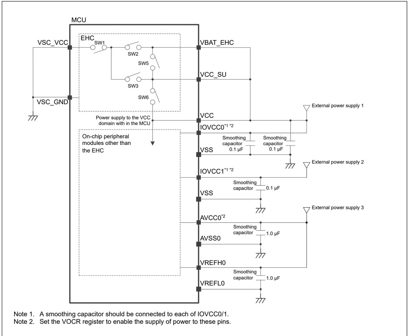
Figure 1.2 Normal startup mode with multiple power sources
