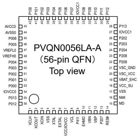
Figure 1.7 Pin assignment for QFN 56-pin
