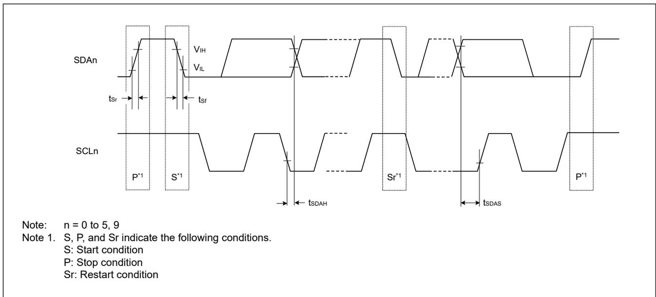
**Figure 2.28 SCK input/output timing (simple I<sup>2</sup>C mode)**
