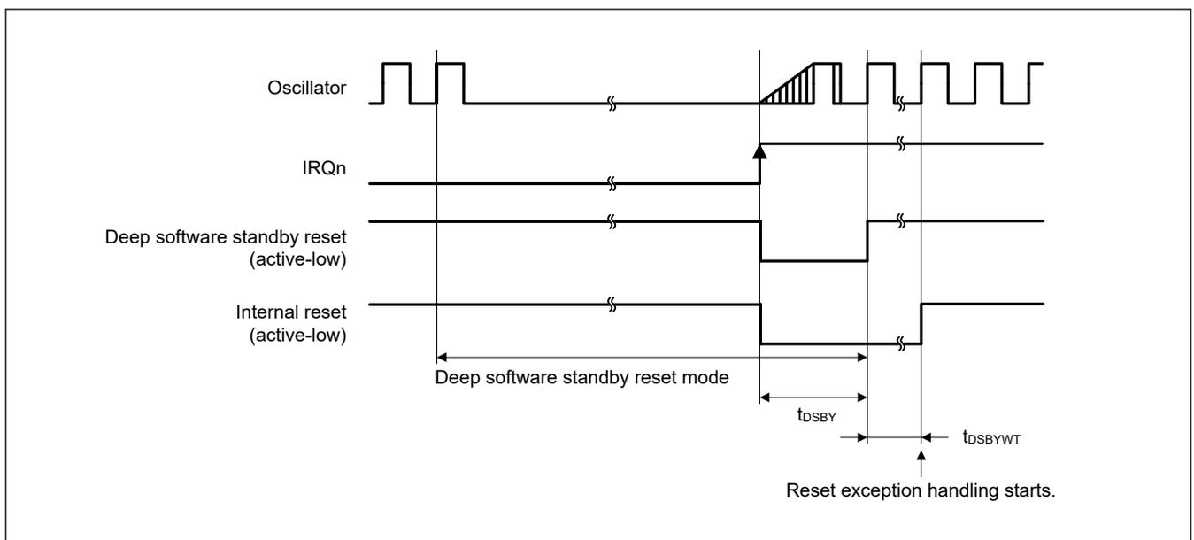
Figure 2.10 Deep software standby mode cancellation timing
