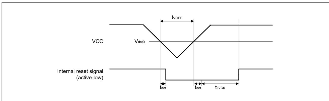
Figure 2.45 Voltage monitoring 0 circuit detection voltage timing ( $V_{det0}$ )
