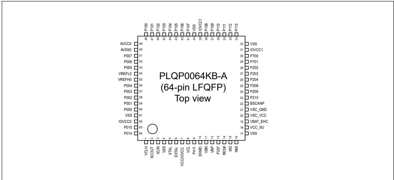
Figure 1.4 Pin assignment for LQFP 64-pin
