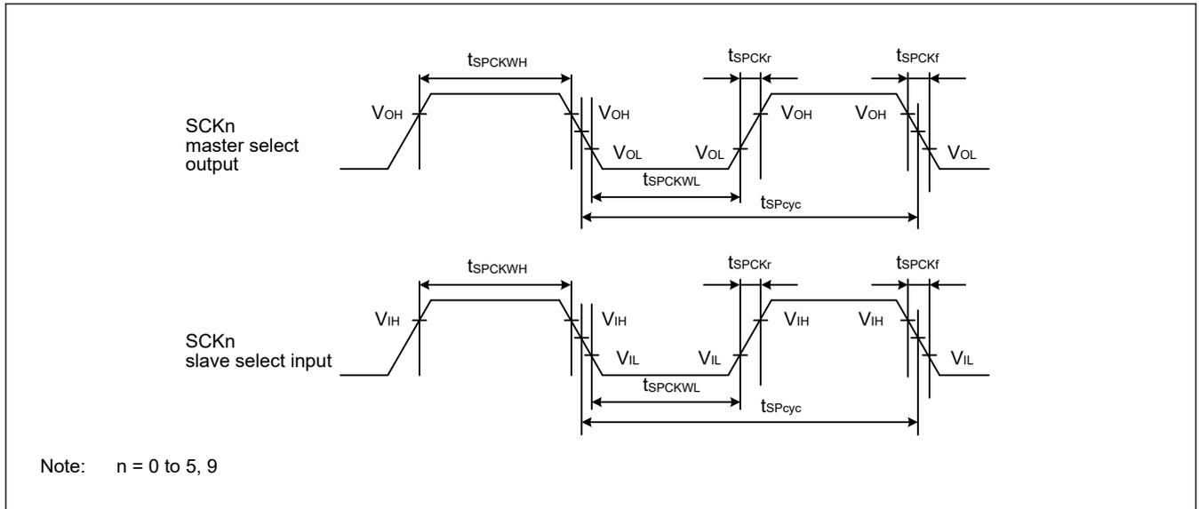
Figure 2.23 SCK clock input/output timing (simple SPI mode)
