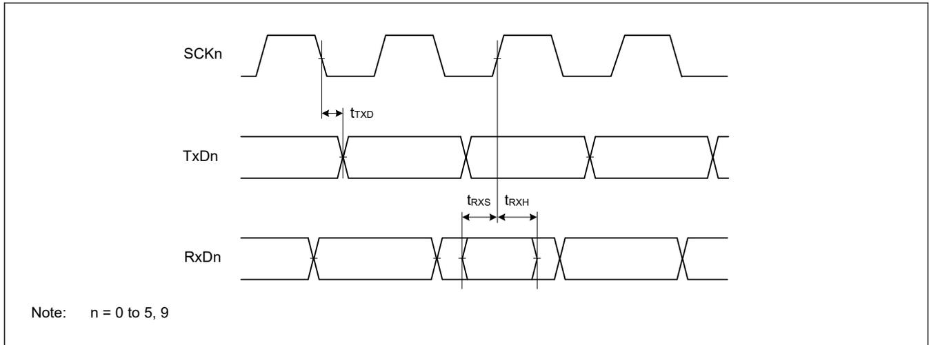
Figure 2.22 SCI input/output timing in clock synchronous mode
