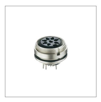
Chassis socket acc. to AISG specification and IEC 61076-2-106, IP68, with threaded joint, for printed circuit boards, for back side mounting
