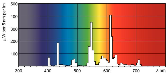
LDPB\_PLL4P\_830-Spectral power distribution B/W
