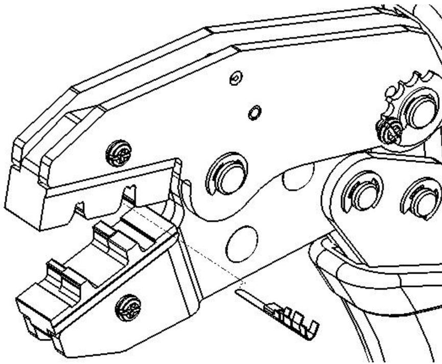
1. First, to place the open barrel into the die set.
