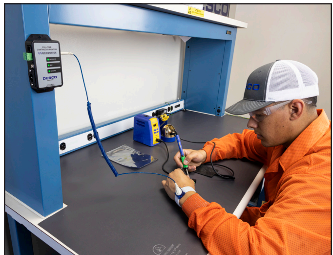
Figure 14. Using the Full-Time Continuous Monitor when mounted on a workbench upright
