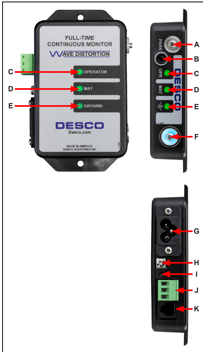
Figure 6. Full-Time Continuous Monitor features and components
