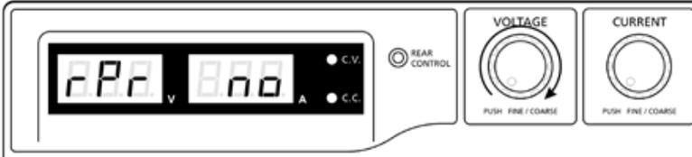
The Current meter is showing “no” at this time. Then rotate Current Control Knob until Current meter showing “YES”.
