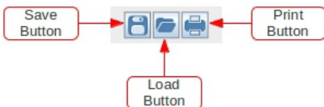
In previous session, the above 3 buttons are used to save, load and print log data. In addition, these buttons can used to save, load and print setting for External Timed Program and Internal Preset Memory.
