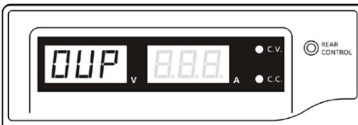
To reset the warning, switch off the unit and remove all loading.
