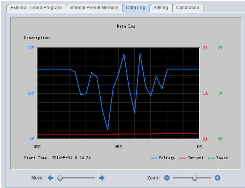
Data log window is used to display output Voltage, Current and Power against time in graphical view.
