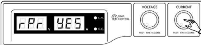
Finally press Voltage Control Knob to exit MENU mode
