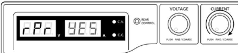
Press Current Control Knob once to confirm. The “YES” will be lighted after preset output being reset to factory default value.
