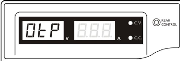
Check your load and output setting. Allow the unit to cool down for at least 30 minutes.
