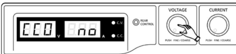
When it is showing “CCO”, rotate Voltage Control Knob until Voltage meter showing “rPr”.
