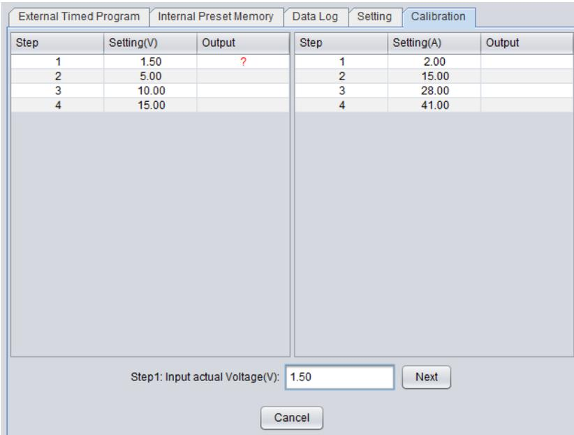
There are total 8 steps for calibration. 4 steps for Voltage and 4 steps for Current. You only need to follow step by step to finish calibration.
