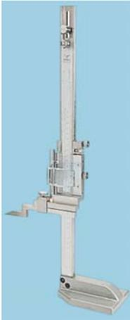
Beam & slide manufactured from hardened stainless steel. The main and vernier scales are satin chrome with the sliding scale raised to prevent wear. The gauge has a fine adjustment mechanism with a carbide tipped scriber. Imperial and metric readings.
