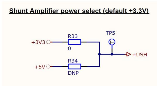
Figure 3: Power supply select for shunt amplifiers
