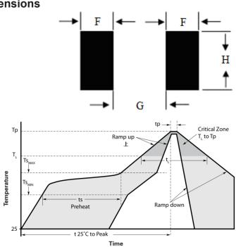
Recommended reflow methods: IR, hot air oven, N2 environment for lead-free.
