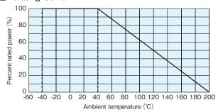
For resistors operated at the ambient temperature of 40°C or higher, the power rating shall be derated in accordance with the above derating curve.
