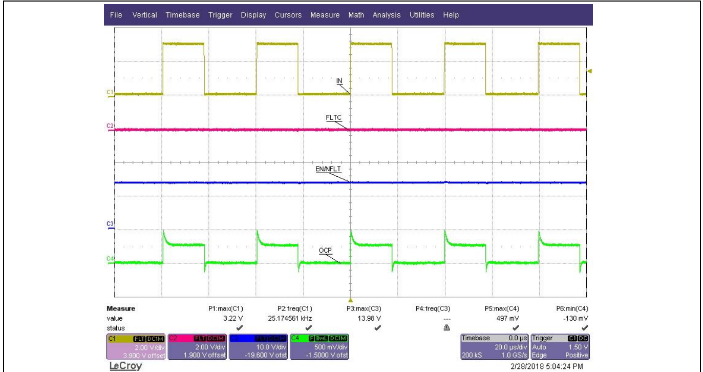
Figure 6 Normal operation (C1: IN, C2:FLTC, C3:EN/NFLT, C4:OCP)
