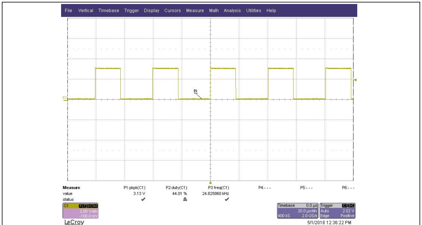
Figure 5 Onboard pulse-signal generator output (C1: IN)
