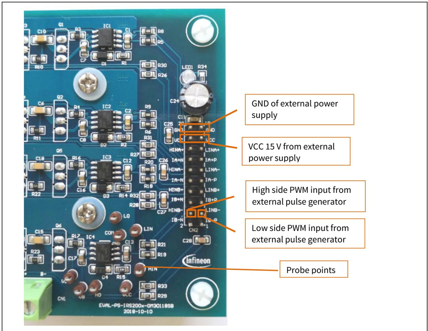
**Figure 4 Evaluate the driver IC on board**
