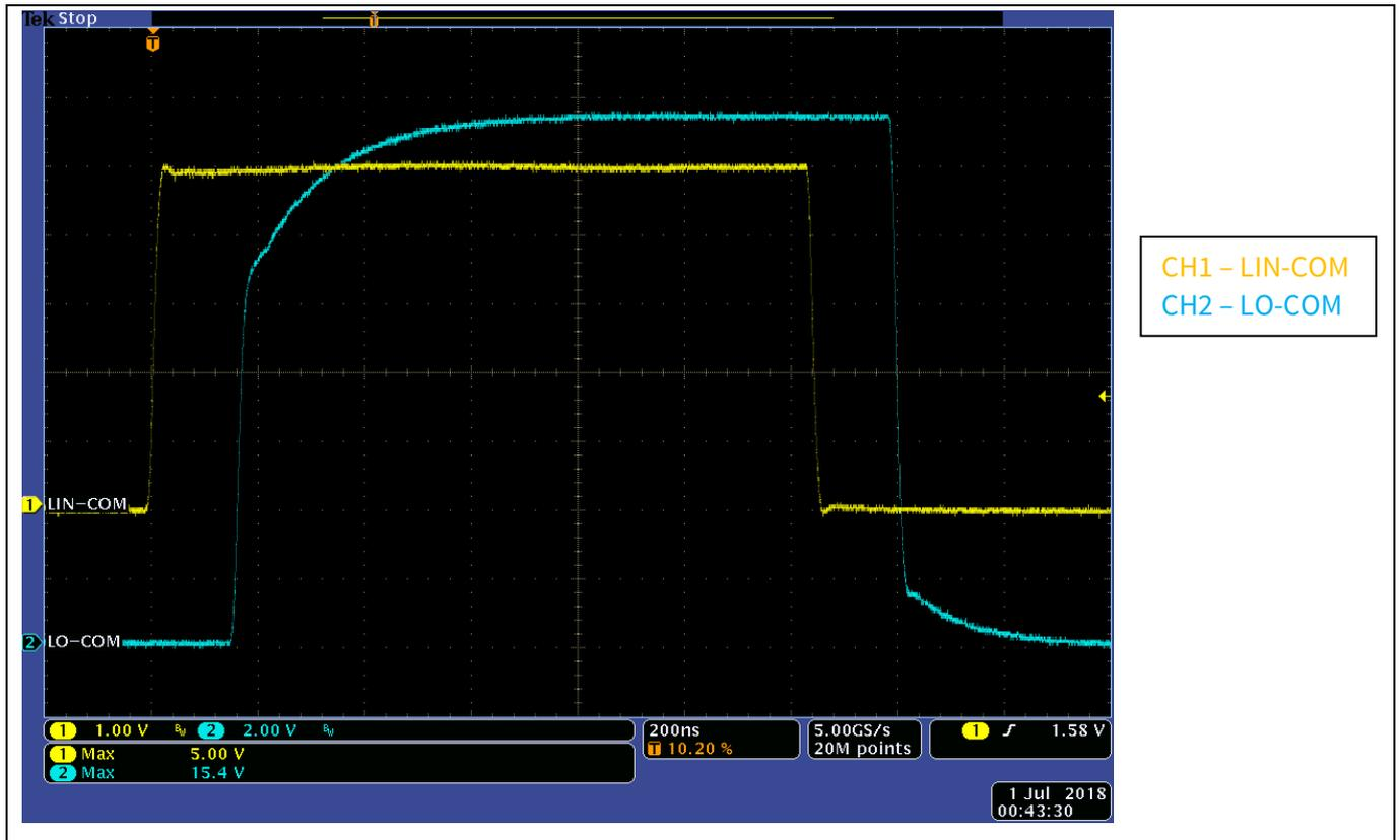
**Figure 5 Typical waveform of driver IC switching performance**
