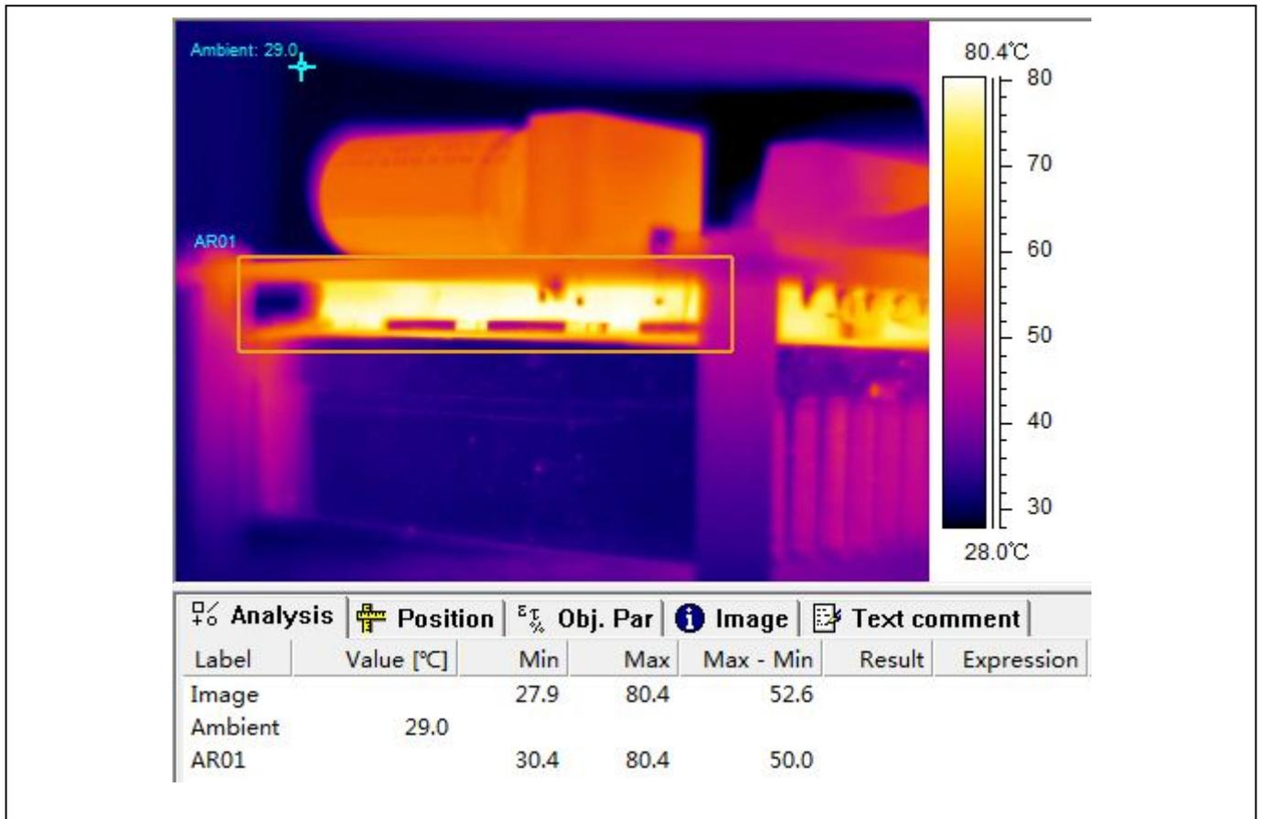
**Figure 10 MOSFET temperature rise at 72 V<sub>DC</sub> input and 7 A<sub>RMS</sub> phase current**
