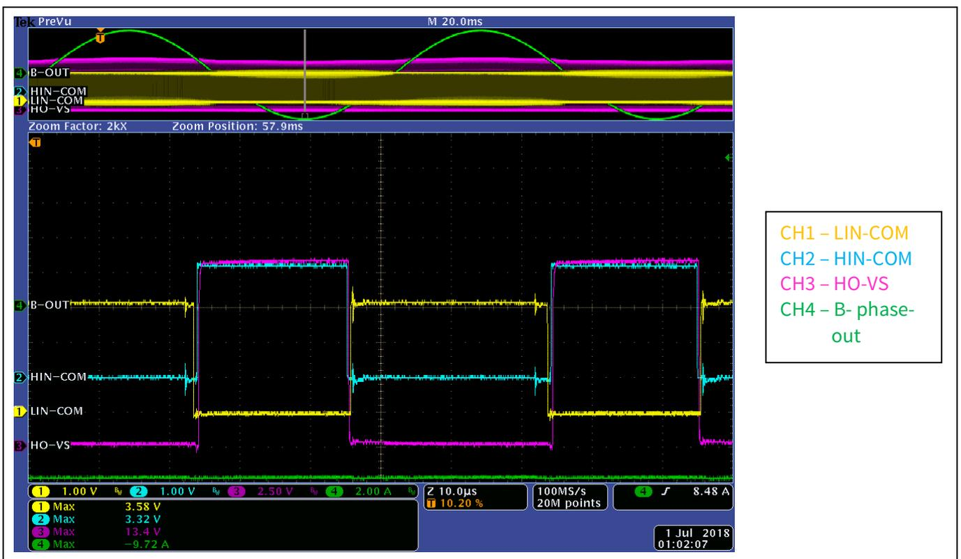
**Figure 7 The input signals probed at 7 A<sub>RMS</sub> phase-out current**
