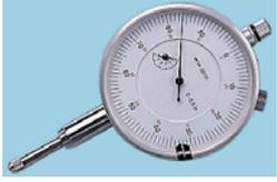
Dial size 60mm/2¼in diameter. Fitted with standard lug back fitting, hardened and ground racks, adjustable dial, bezel lock and tolerance pointers.
