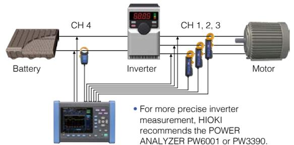
• For more precise inverter measurement, HIOKI recommends the POWER ANALYZER PW6001 or PW3390.
