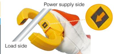
For example, you won't be able to measure power or power factor accurately if the clamp is oriented incorrectly.
