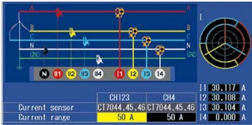
**STEP 3** The instrument will perform an automatic wiring check and display the results.
