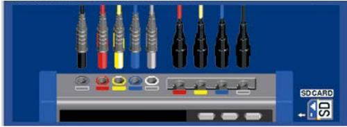
**STEP 2** Connect the voltage cables and current sensors to the circuit to be measured.
