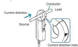
If attached with the current direction indicator pointed in the opposite direction of the current, the phase is displayed deviating by 180 degrees. 5 Make sure the jaw is firmly closed.
