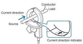
If the clamp is attached with the current direction indicator pointed in the opposite direction of the current, the phase is displayed deviating by 180 degrees.
