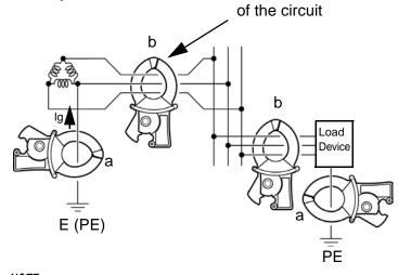
Three-phase 3-lead circuits Clamp all three leads
