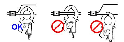
When making the phases of the measurement current and output voltage the same, clamp the jaws of the sensor onto the conductor so that the current direction on the clamp points in the direction of the load, and so that the conductor is approximately centered between the jaws. Make sure that the tips of jaws are fully closed.
