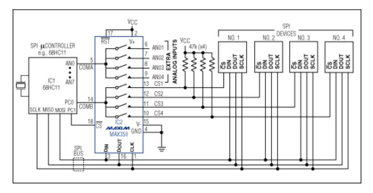
A dual 4-channel multiplexer expands the number of input channels and chip-select lines that this microcontroller can support.
