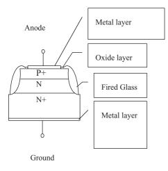
The p-n junction diode is a unidirectional device. For use on AC signal lines, bi-directional devices are available which are based upon stacking two diodes back to back. Most manufactures use monolithic NPN and PNP structures. The center region is made relatively wide compared to a base of transistor to minimize the transistor action which can cause increased leakage current.
