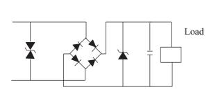
Transient Voltage Suppressors 1 shown in figure 4 provides a maximum protection. However, we do not recommend to use the TVS diode here, unless we can know the electric circuit impedance and the magnitude of surge rushed into the circuit. Otherwise the TVS diode is easy to be destroyed by voltage surge.
