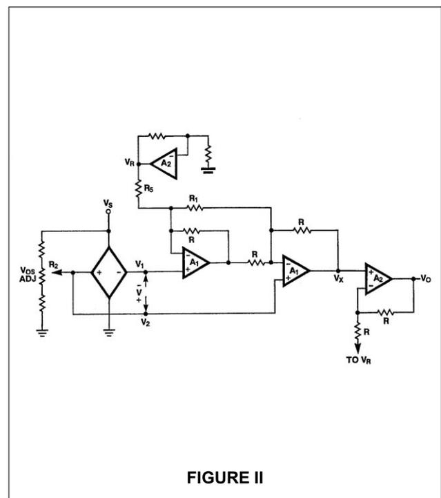
Neglecting the small error terms of the op amps, the equation for the first stage output voltage,  $V_X$  in terms of the bridge arm voltages,  $V_1$  and  $V_2$ , is given by
