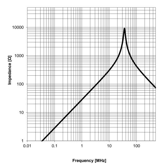
GENERAL TOLERANCE PROJECTION METHOD CREATED CHECKED Würth Elektronik eiSos GmbH & Co. KG **EMC & Inductive Solutions** KaS BMoe DIN ISO 2768-1m Max-Eyth-Str. 1 74638 Waldenburg **WE-MAIA SMD Power Inductor** Tel. +49 (0) 79 42 945 - 0 ORDER CODE www.we-online.com 78438324047 eiSos@we-online.com DATE (YYYY-MM-DD) BUSINESS UNIT REVISION STATUS PAGE 001.002 Valid 3/7 2512 2017-04-17 eiSos **WÜRTH ELEKTRONİK**
