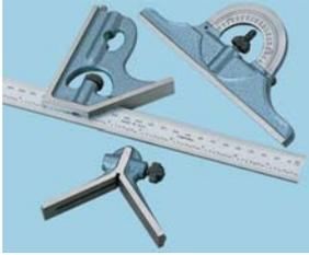
The square and centre heads are of hardened steel. Protractor head is reversible and is graduated 0° to 180° in both directions. All heads have blue stove enamelled hammer finish with accurately ground working surfaces. The 300mm/12in blade is fully tempered and hardened. Satin chrome finish gives exceptional clarity to the very fine graduations and resists abrasion.
