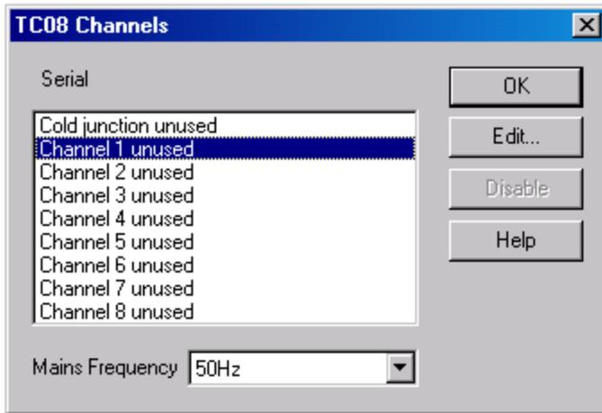
8. In the TC-08 Channels window, double-click on **Channel 1 unused**. The Edit TC-08 Channel dialog box appears.
