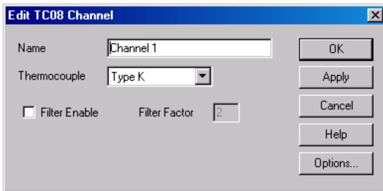
9. From the **Thermocouple** drop-down list, select the type of thermocouple you are using and click the **OK** button. The TC-08 Channels dialog box reappears.
