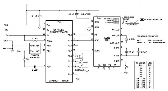
Figure 8. Application using SDIO pins.
