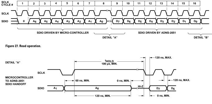
Figure 28. Microcontroller to ADNS-2051 SDIO handoff.
