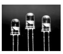
The AlInGaP II technology provides extremely stable light output over very long periods of time, with low power consumption.
