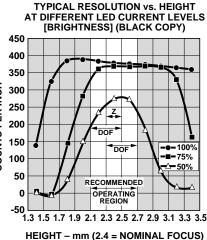
Figure 24. Typical resolution vs. z (black copy and LED variation).<sup>[2,3]</sup>
