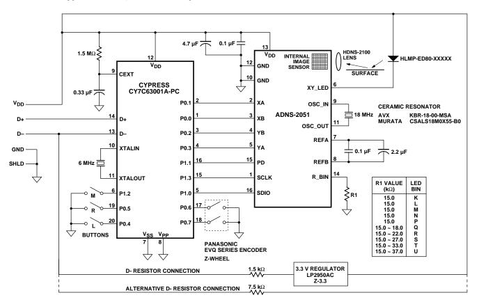
Figure 9. Application using quadrature output pins.
