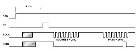
Figure 37. Power up serial port PD sync sequence.
