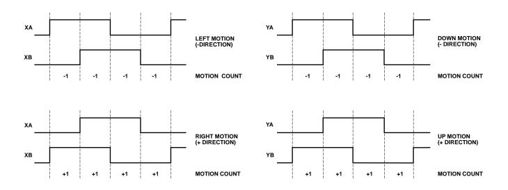
Figure 20. Quadrature output waveform.
