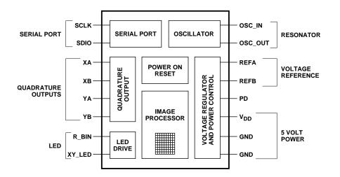
Figure 6. Block diagram of ADNS-2051 optical mouse sensor.
