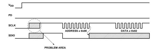
Figure 35. Power up serial port watchdog timer sequence.
