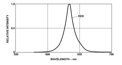
Figure 1. Relative Intensity vs. Peak Wavelength.
