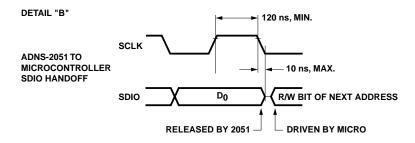
Figure 29. ADNS-2051 to microcontroller SDIO handoff.
