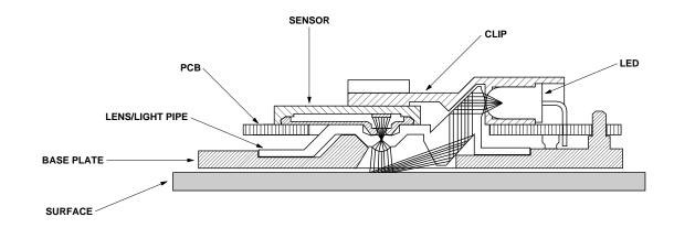
Figure 7. PCB assembly.
