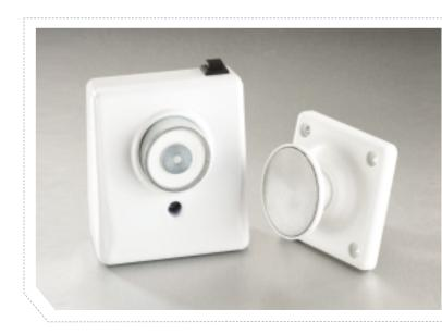
Electromagnetic Fire Door Holders are designed to hold open Fire Doors in any areas where easy access is essential, and can be used in conjunction with any suitable fire alarm systems. When an alarm is triggered, power to the door holder is cut, allowing the fire door fitted with it's standard closing mechanism, to shut automatically. Type 87 door holders are fitted with an integral manual release button, allowing the door to be closed without operating the fire alarm.
