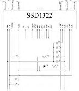
MCU Interface Selection: BS0 and BS1 Pins connected to MCU interface: D7~D0, E/RD#, R/W#, D/C#, CS#, and RES#
