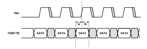
Figure 14. HDMP-1512 (Transmitter) Timing Diagram, with PPSEL = 0.
