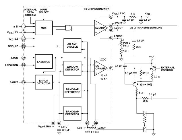
Figure 3. Laser Driver Block Diagram and External Circuitry.
