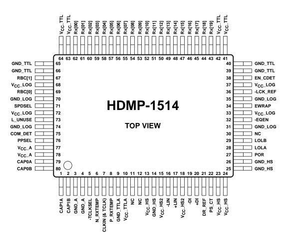
Figure 12. HDMP-1514 (Rx) Package Layout.
