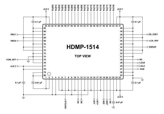
Figure 21. Typical Receiver Pin Terminations for Applications Using High Speed Fiber Links ( $\pm$  DIN). For 1062.5 MBd Operation Only, SPDSEL (pin 71) Set High, Non Ping-Pong Mode (PPSEL = 0).
