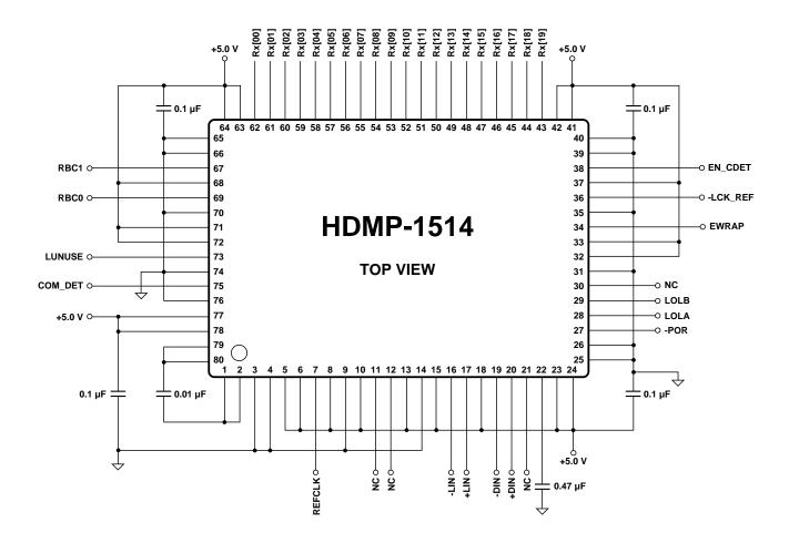
Figure 20. Typical Receiver Pin Terminations for Applications Using High Speed Serial Copper Links ( $\pm$  DIN). For 1062.5 MBd Operation Only, SPDSEL (pin 71) Set High, Non Ping-Pong Mode (PPSEL = 0).
