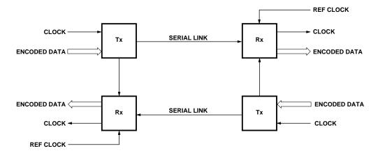
Figure 1. Point-to-Point Data Link.
