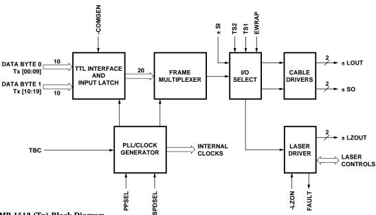
Figure 2. HDMP-1512 (Tx) Block Diagram.
