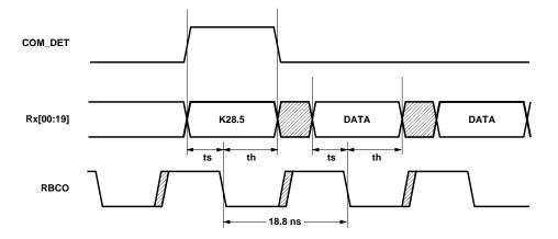
Figure 15. HDMP-1514 (Receiver) Timing Diagram, with PPSEL = 0.
