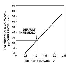
Figure 8. Typical Plot of Loss of Light Threshold Voltage vs. DR\_REF Voltage.
