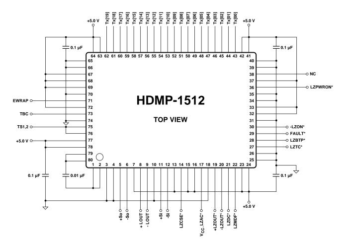
Figure 19. Typical Transmitter Pin Terminations for Applications Using the On-Chip Laser Driver. For Details of the Laser Driver Connections, Indicated by "\*," see Figure 3 on page 4. For 1062.5 MBd Operation Only, SPDSEL (pin 67) Set High, Non Ping-Pong Mode (PPSEL = 0).
