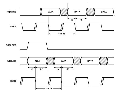
$Figure\ 17.\ HDMP-1514\ (Receiver)\ Timing\ Diagram\ in\ Ping-Pong\ Mode,\ with\ PPSEL=1.$
