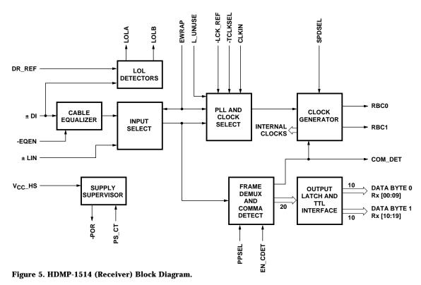
path using the -EQEN pin, # 32. Setting pin #32 high disables the equalizer. Setting pin # 32 low enables the equalizer. The typical performance of the input equalizer is shown in the (frequency response) plot of Figure 7. The impact of the equalizer is improved BER performance over long lengths of cable (10 to 20 meters).
