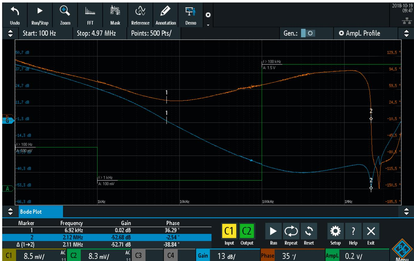
The R&S®RTA-K36 frequency response analysis (Bode plot) option characterizes the frequency response of a variety of electronic devices, including passive filters and amplifier circuits
