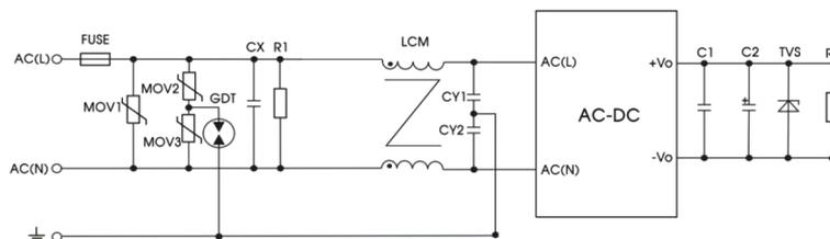
Fig 2: EMC application circuit with higher requirements
