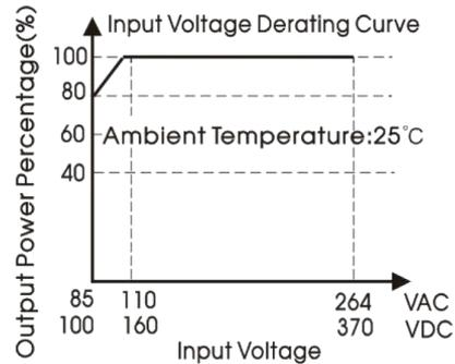
Note: ① With an AC input between 85-110VAC and a DC input between 100-160VDC, the output power must be derated as per temperature derating curves;
